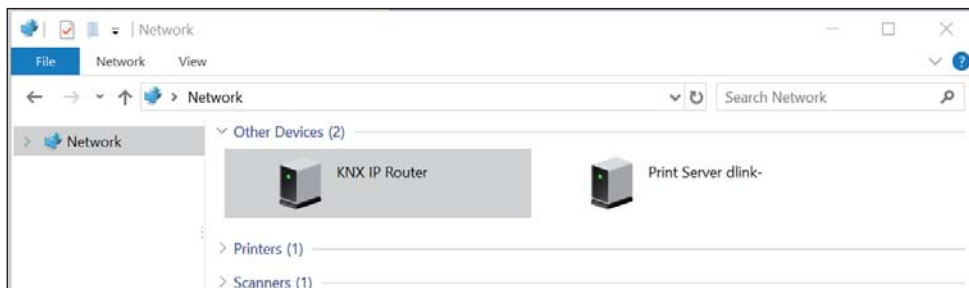
Figure 13: KSR-01IP as UPnP network device (“KNX TP IP”)
